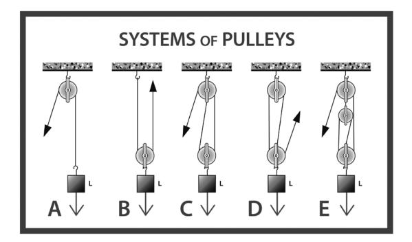
A rope and pulley system –that is, a block and tackle– is characterized by the use of a single continuous rope to transmit a tension force around one or more pulleys to lift or move a load–the rope may be a light line or a strong cable.
