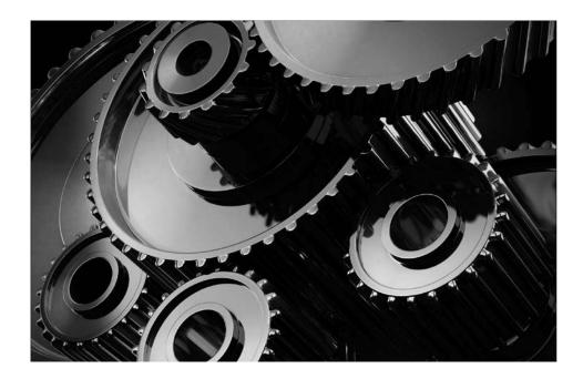
A gear or cogwheel is a rotating machine part having cut teeth, or cogs, which mesh with another toothed art to transmit torque, in most cases with teeth on the one gear being of identical shape and often also with that shape on the other gear. Two or more gears working in a sequence (train) are called a gear train or, in many cases, a transmission; such gear arrangements can produce a mechanical advantage through a gear ratio and thus may be considered a simple machine.
